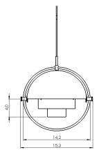
MEASUREMENT - L x W x H inches Lamp height: 14,2 inches Lamp diameter: dia. 14,2 inches canopy size: dia. 4,5 x 2,3 inches Wire length, exposed: Approx.. 157,5 inches
